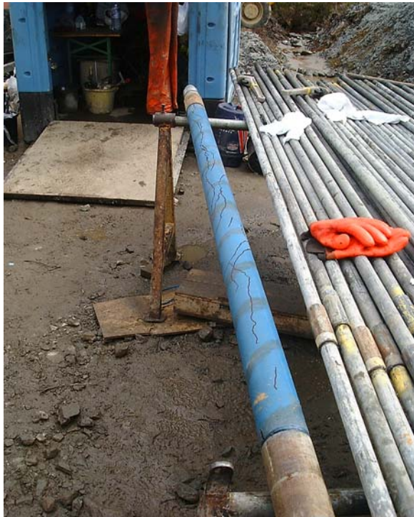
Figure 2.3 – Impression packer recovered from BH PT3A at 279.5 m depth with fractures traces marked up with felt tip pen.
